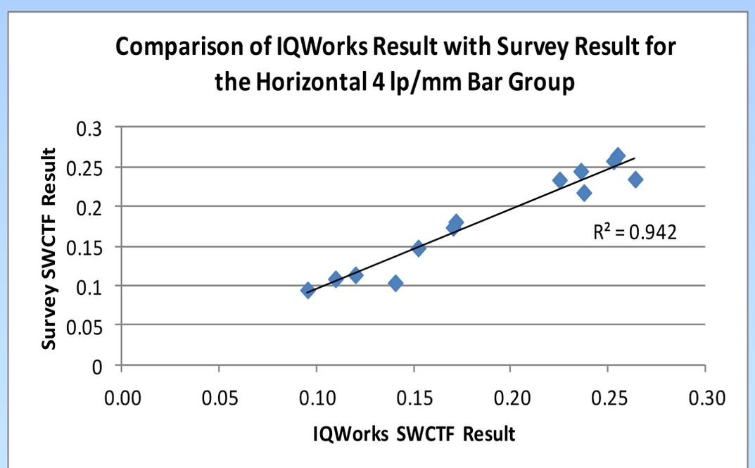
Figure 3—Comparison of IQWorks SWCTF result with SWCTF result acquired during survey by using ROI tools at console workstation. Graph shows a good agreement between both methods.
