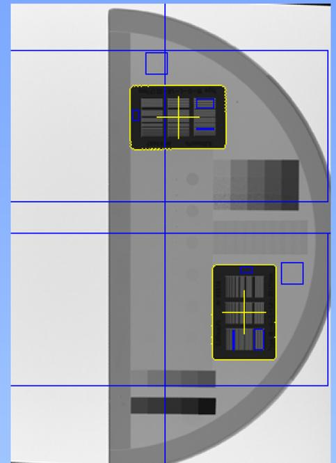
Figure 2—Screen shot showing the analysis tree applied to an image of the test object. Yellow lines indicate bar group sets detected by the edge detect modules and blue lines represent ROI's automatically positioned relative to the detected bar group sets.
