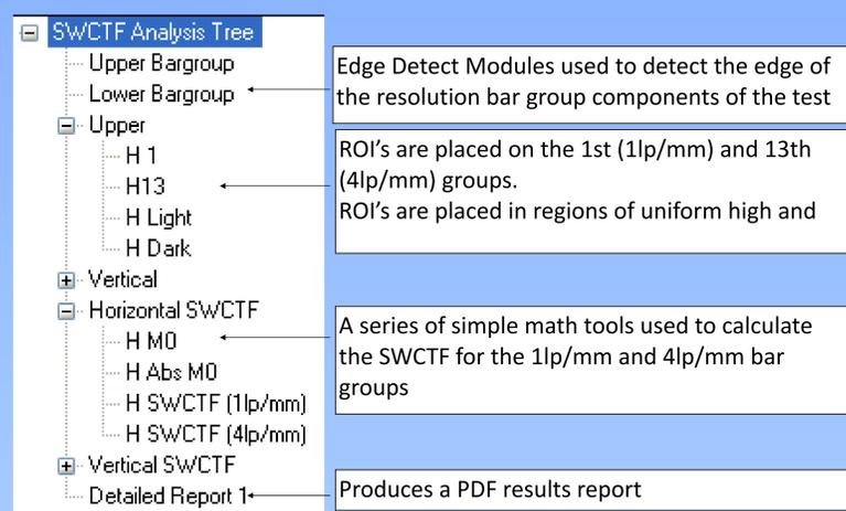
Figure 1—Schematic of analysis tree created to calculate SWCTF for both sets of bar groups in both the horizontal and vertical gratings. The vertical components of the analysis tree have been minimised for illustration.
